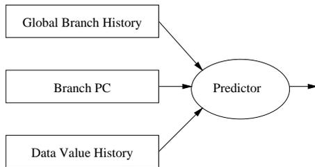
**Fig. 2. Using data values for branch prediction directly.**
